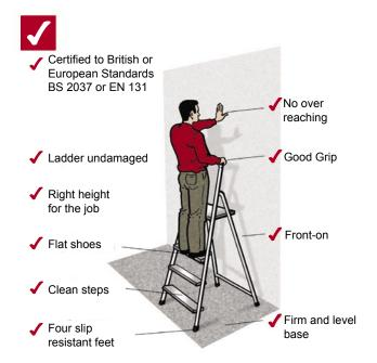
A step ladder is an important piece of equipment. Used correctly and safely a Youngman step ladder will provide many years of reliable use.
