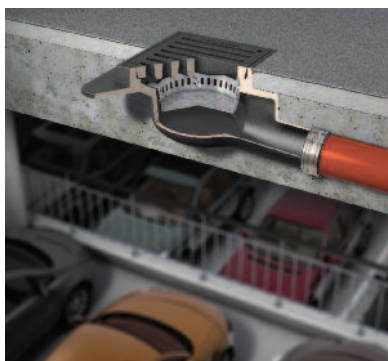
Shallow deck installation with 110mm horizontal outlet with weep-hole drainage facility. Complete with locked grating and galvanised steel dirt bucket.
