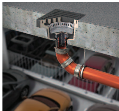
Through deck installation with 110mm vertical outlet complete with locked grating, galvanised steel dirt bucket and R120/2 hour fire stop cartridge fitted.
