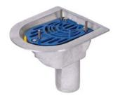
ACO Balcony outlets are designed to be installed against an abutment wall and permit the introduction of successive rainwater pipes discharging from higher level balcony areas. Balcony outlets are suitable for connection to pipes of 82.5mm and 110mm outside pipe diameters.
