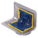
ACO Two Way outlets are located at the junction between flat roof and parapet wall providing "through the wall" drainage to external rainwater pipes and hoppers. Outlets are parallel threaded for connection to taper male, screw threaded adapters to ensure a completely watertight connection to pipes with 55mm, 82.5mm and 110mm outside pipe diameters.
