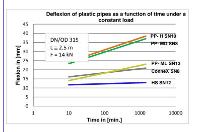
For the nominal diameters < DN/OD 250 and > DN/OD 500, longitudinal flexural strength values can be calculated for both the HS and CONNEX pipes on the basis of the experimental results.
