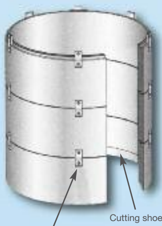
Bolt and jointing plates
