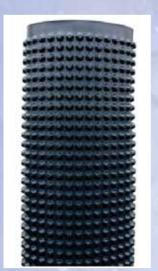
Protecto-drain 20 is a 1mm thick HDPE membrane which is useful for larger scale areas of tanking and sealing. It has a larger cup size of 20mm which allows a greater amount of ground water to pass along the membrane.
