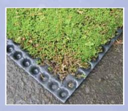
Protecto-drain 20P was developed for use as a reservoir and drainage layer in green roof construction. It is placed on top of the waterproofed, protected concrete deck and sits beneath a filter layer, the soil substrate and vegetation layers on extensive green roof systems.
