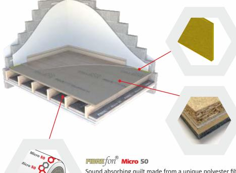
DECKfon<sup>®</sup> **Quattro 39** Acoustic overlay board designed for direct to joist refurb timber floor applications
