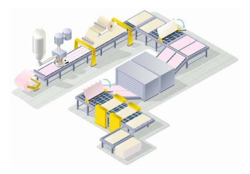
The initial materials are homogenously mixed to form a gypsum slurry that is spread via multiple hose outlets onto a paper liner on a moving belt conveyor. A second paper liner is fed onto the production line from above to form the plasterboard. The plasterboard continues along the production line where it is finished, dried, and cut to size.
