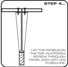
\* When using larger chipboard sheets, for added stability, fix additional Loft Leg XLs around the perimeter of the storage deck. See diagram overleaf. IMPORTANT:
