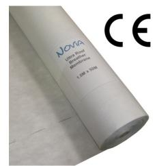
An ultra-low cost, entry grade synthetic 3 layer laminate utilising an advanced microporous breathable polymer. The roll is grey in colour, with no print or logo, apart from installation lap lines. This 100gsm dual CE Approved breather membrane is commonly used for timber frame constructions.
