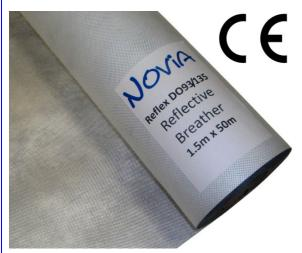
A reflective breather membrane which is suitable for all under-slating or under-cladding timber frame applications. Grade DO93/135 is a metallised-faced laminate of non-woven fabrics with high water resistance and good vapour permeability, which is also flame-resistant to EN 13501-1 grade E. The material has low emissivity and high reflectivity for improved performance over and above that of the standard breather.
