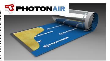
A 33mm air-open reflective insulating breather membrane made with high density glasswool encapsulated between a perforated reflective lower layer and Klober Permo® air. PhotonAir is water tight and upgrades thermal insulation without the risk of condensation.
