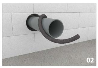
• Apply a PU joint filler around the PVC pipe for half the thickness of the wall.
