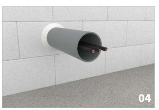
• Pull the cables through the pipe.
