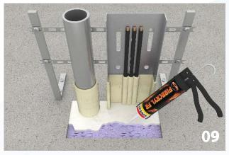
• Apply a layer of Firecryl FR of 4mm on both sides of the opening.
