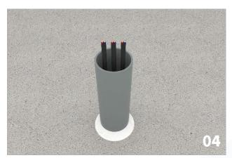
• Pull the cables through the pipe.
