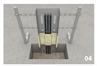
• Apply a piece of cardboard with PE foil below the opening.
