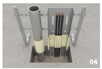
• Apply a PU joint filler around the PVC pipe for half the thickness of the floor.
