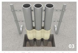
• Apply a layer of Fire Blanket covering the cables for a length of 23cm from the wall, on both sides of the ceiling.
