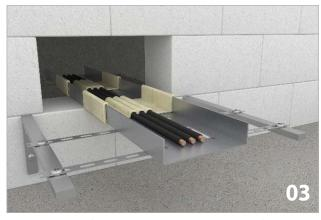
• Apply a layer of Fire Blanket covering the cables for a length of 23cm from the wall, on both sides of the wall.
